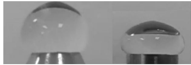
FIGURE 13. Comparison of two drop volumes, the drops grow with different boundary conditions on walls tube.
