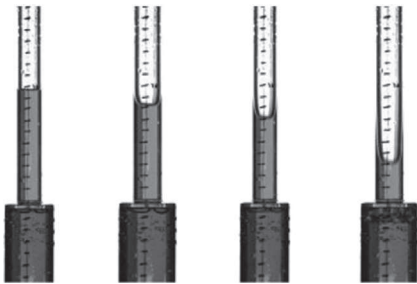
Fig. 6: Snapshots of the gravity-induced flow in concentric pipes. In this case \alpha = 0.178 and \beta = 0.833 . Pipes were filled with ethanol. Times from left to right are t = 0, 11/500, 16/500 and 27/500 s.
